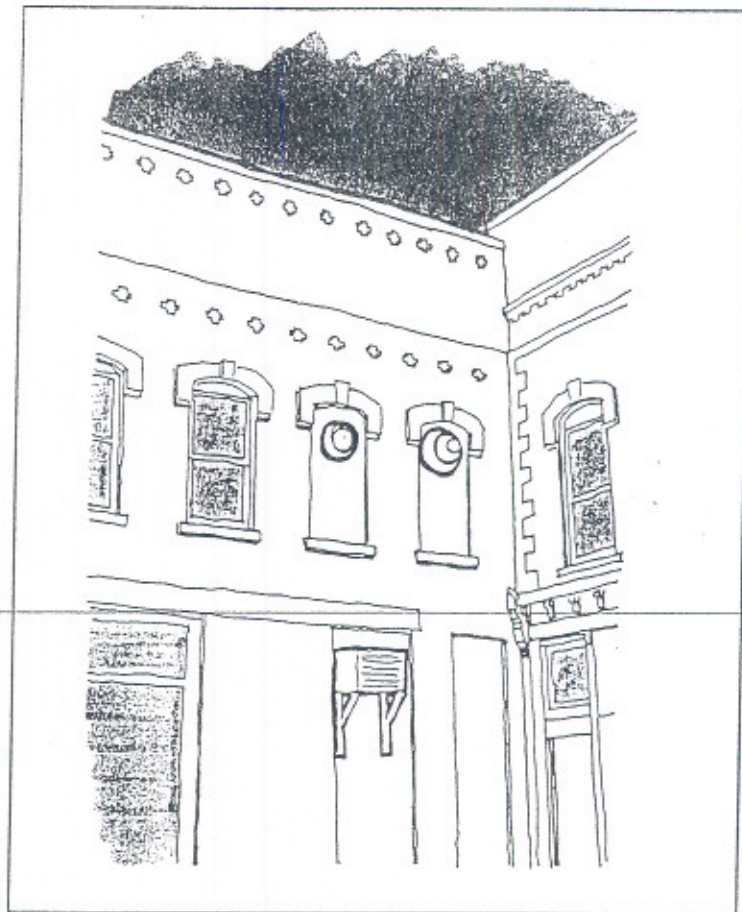
Fig. 2.12.1 Exposed mechanical equipment detracts from streetscape appearance
