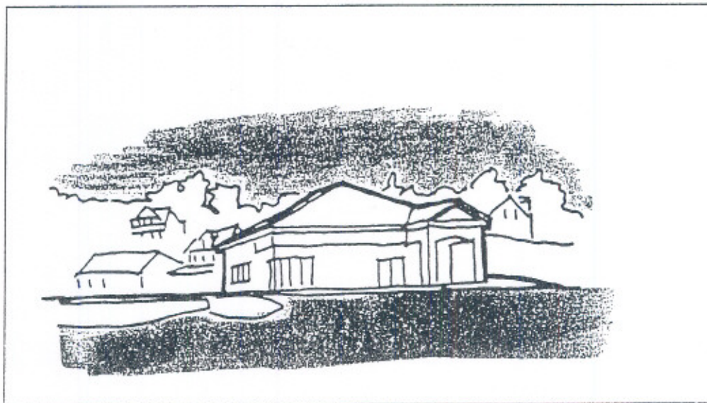
Fig. 2.4.4 A simple change of roof can improve the integration with the community
