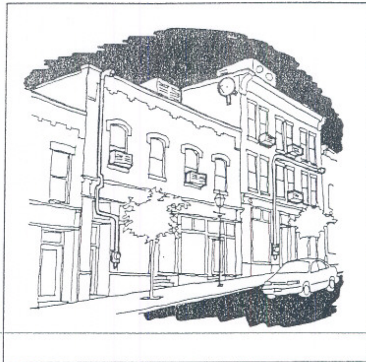
Fig. 2.12.2 Visible mechanical and electrical equipment should be relocated or concealed...
