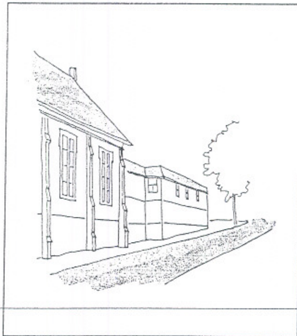
Fig. 2.9.1 Building addition and roof not related to existing building
